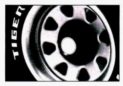
If the wheel has a plastic center cap, you do not have to remove the center cap to loosen the wheel nuts.
